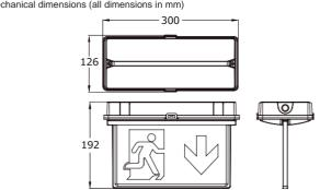
BY-B2136E exit signal can be installed on ceilings. It is particularly suitable for outdoors such as offices, schools, universities and hospitals. It incorporates a green LED indicator that shows battery charging mode. Safety and performance according to EN 55015, EN 61347, EN 60598-1, EN 60598-2-22, EN 61000-3-2, EN 61000-3-3. The built-in battery unit ensures an emergency operation period higher than 3 hours.
