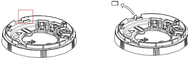
8. To detach a locked sounder, insert the key included with the base into base's keyhole and turn it 180° clockwise. Then, rotate the sounder head counterclockwise to release it from the base.
