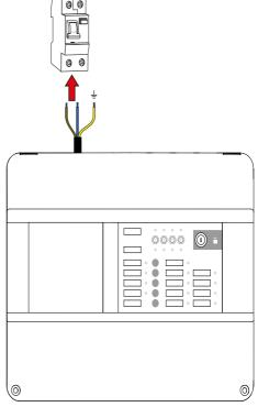
To ensure that the mains cable is securely attached, insert the cable into the plastic guide, using the tabs in the housing. This will prevent the cable from coming loose in the event of sudden removal.
