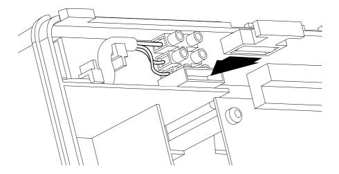
**NOTE:** Never use the fuse from the mains terminal block as a switch to connect and disconnectthe control panel from the mains. Use the circuit breaker's lever.
