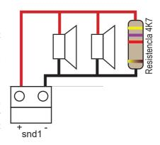
According to the standards, it is not permitted to make a star-connected wire shunt or install the end-of-line resistor on the terminal block if the sounder output is in use.
