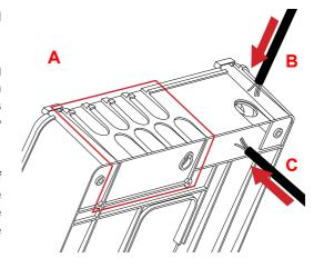
**CAUTION:** Be careful when drilling the housing to make a hole for the lines, you may damage the control panel's electronics.
