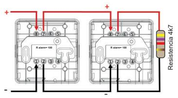
Manual call point must be installed at a height of between 1.2 and 1.5 m from the floor and be clearly visible, properlylabelled and accessible. If the manual call points of another manufacturer are used, check that they are compatible, e.g. check that they use an alarm level resistor. Otherwise, it will have to be added (the value of this resistor is 100 ohms 2W).
