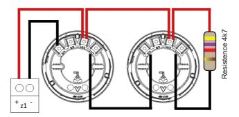
As shown in the above drawing, the + is connected to contact no. 1 (through which is enters and leaves), while the negative terminal is connected with the line entering through contact no. 4 and leaving through contact no. 3 to the following detector. At the end of the lineyou must place a 4K7
