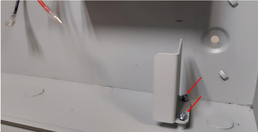
Figure 7: Battery Holder Brackets
