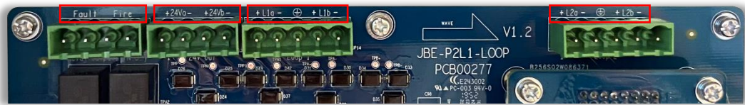
Figure 4: Loop Board Connections
