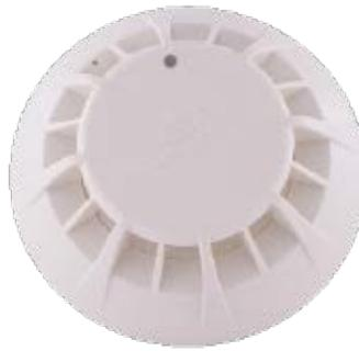
JBE-2107 is a conventional heat detector designed to operate on a zone line of conventional intelligent fire detection and alarm devices. This heat detector sends fire alarm signals to the fire panel when the air temperature (or its rate of rise) reaches the alarm thresholds defined in the European norm EN 54-5.
