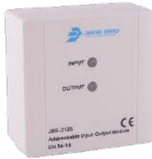
JBE-2125 is an addressable output module with one feedback input designed to operate on a loop of intelligent fire detection and alarm devices with the JBE loop protocol.
