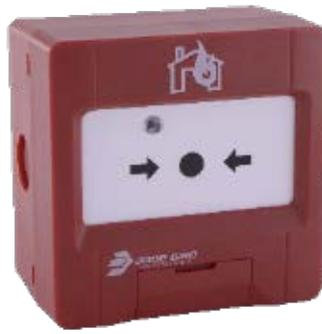
JBE-2101 is a conventional manual call point (MCP) designed to be compatible with a wide range of conventional fire panels and input modules. This MCP sets an installer-selectable resistive load to the fire zone when its resettable element is pressed.
